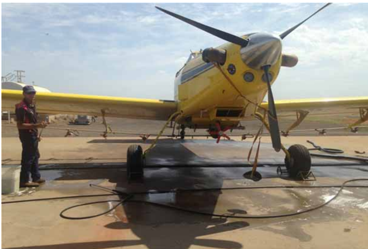
Figure 2: Appropriate wash-down area with culvert to collect run-off into a catchment area (Photo: Nina Sheer, EPA)
